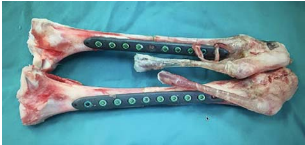
Figure 1. Tibial bone fracture after fixation with an implant devoid of a threaded plug and additional threaded plug in the hole at the level of fracture in group 2 and group 3 respectively
